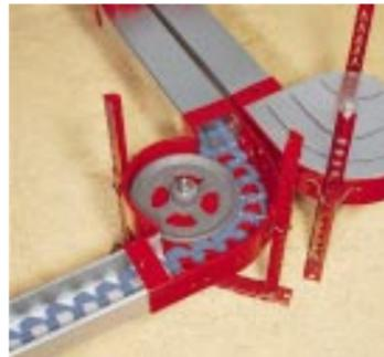
Completely enclosed in a powder coated, steel housing, the corner mechanism is specifically designed for low maintenance and high performance. Mounted on a hardened steel base plate, the corner guide rail and fluted wheel provide maximum wear resistance while assuring smooth chain movement.
