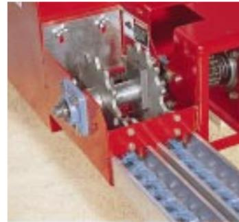
The traditional yoke weldment connecting the drive gears to the motor (an annoying source of shearing and misalignment in chain feeder systems) has been eliminated and replaced by a precision-machined design that reduces the number of parts, guarantees proper alignment and significantly enhances dependability.
